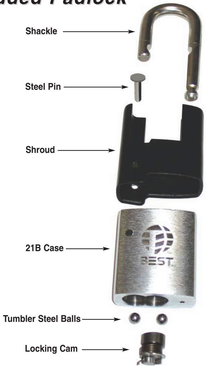
Exploded View 21B Shrouded Padlock
