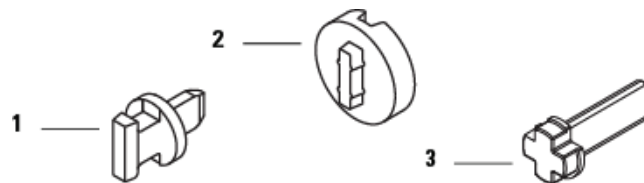
Figure 2.41 Lever components with interchangeable cores
