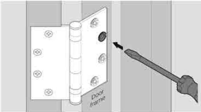
Determine which hinge needs adjustment to allow the door to hang properly in the door frame. Loosen but do not remove the screws from the hinge. For best results; only back out screws two turns.
