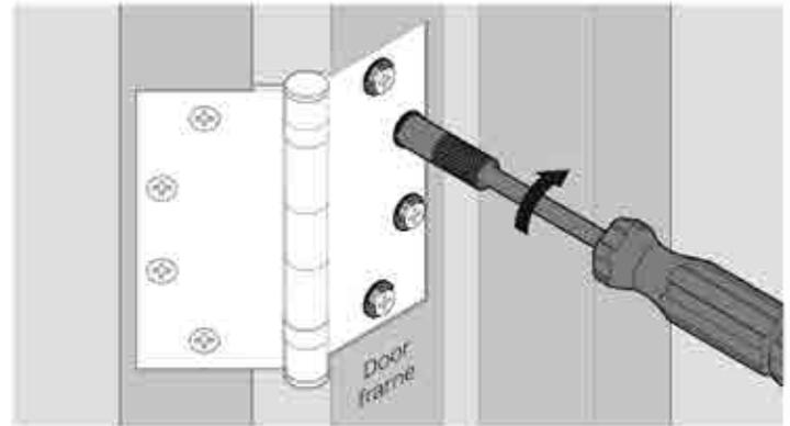
Insert screwdriver through adjustment tool. Slide adjustment tool down to position onto the quick shim adjustable collar and turn the collar to make appropriate adjustment. Once adjustment is complete, simply tighten the screws. Repeat if alignment needs further adjustment.
