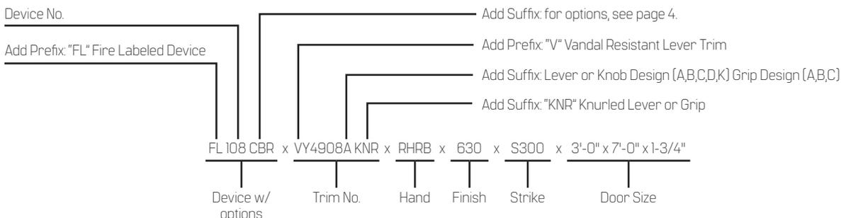
**Device Only:** Device no, hand, finish, strike, and door size including thickness. (e.g. FL108 x RHRB x 630 x S300 x 3'-0" x 7'-0" x 1-3/4")
