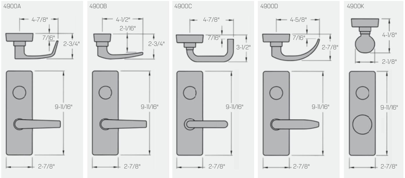
Lever Centerline 38-3/16" from Finish Floor when Device Centerline is 39-15/16".
