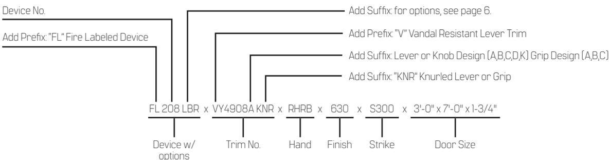
**Device Only:** Device no, hand, finish, strike, and door size including thickness (e.g. FL208CD x RHRB x 630 x 3'-0" x 7'-0" x 1-3/4")
