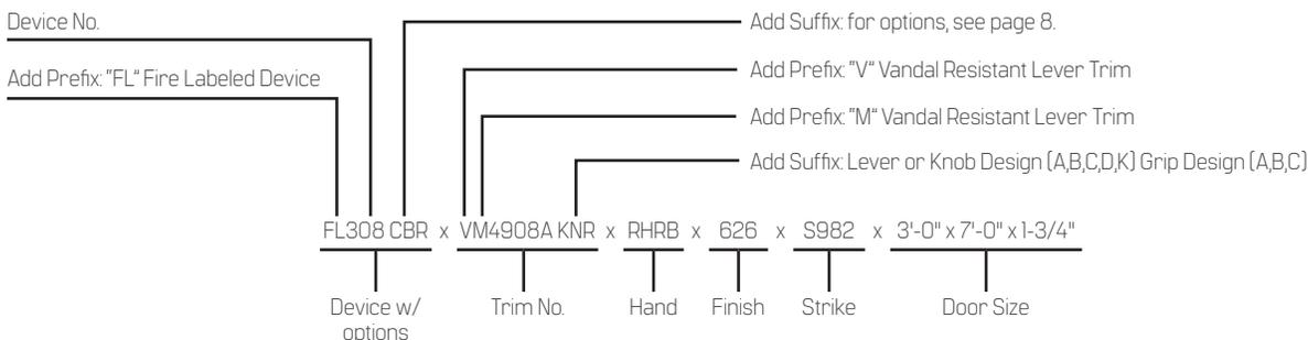
**Device Only:** Device no., hand, finish, strike, and door size including thickness: (e.g. FL308CD x RHRB x 626 x S982 x 3'-0" x 7'-0" x 1-3/4")
